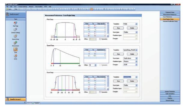
The user can select different scan speeds or data point densities in different regions of the scan, thus optimizing the overall measurement
