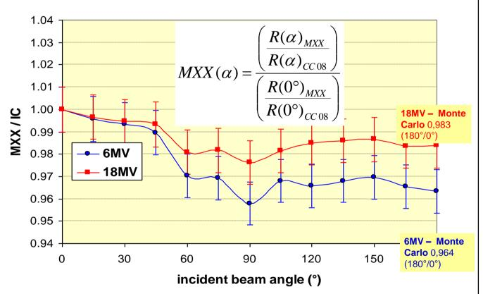
The angular dependency has proven to be more pronounced for low energy but the signal decrease has been found acceptable without any further correction for rotational type of beam delivery.
