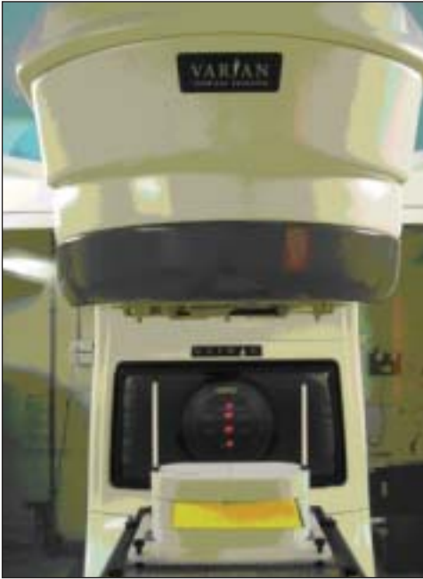
Figure 4: Planar dose distribution measurement setup to expose Kodak EDR2 films. Where the film to Source distance is 100 cm and Phantom surface to Film distance is 5 cm
